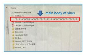
By opening the hidden file instead of the shortcut in the infected USB flash drive, you might be able to find the original file. In this case, the body of the virus exists in the hidden folder, and if the shortcut is opened, the effect the virus is triggered.
